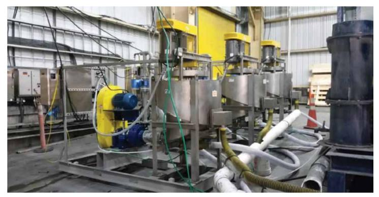
Figure 3: A train of three 0.6-metre StackCells used in this evaluation.
