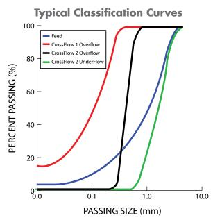
This graph shows the typical size distributions generated during normal operations using two CrossFlow Separators in series to produce 3 tightly-sized product streams for a frac-sand application.
