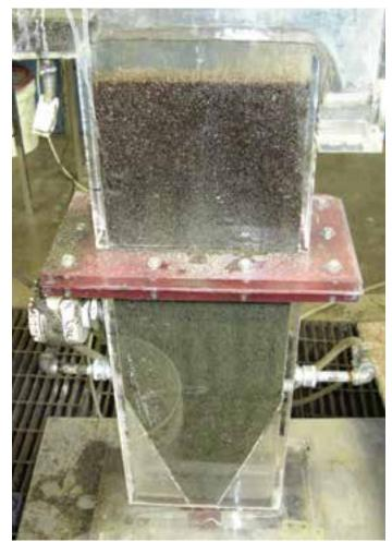
Lab test showing highly efficient teeter-bed separation.
