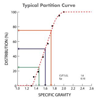
Partition curve from an industrial unit showing a low gravity cut  $(SG_{50})$  and efficient separation of rock from a coal feed stock.
