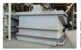
2.2x2.2 meter (7x7 ft) CrossFlow Separator for the recovery of fine tungsten.
