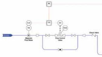
Traditionally, particle size and/or density cut-point has been controlled by adjusting only the fluidization flow rate and the relative level of the teeter bed. More recently, Eriez engineered a superior control system that improves metallurgical results by regulating the true density of the teeter bed through continuous measurements of differential pressure.
