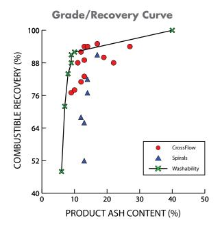
Comparison of teeter-bed separator to spiral concentrator for upgrading 2.0x0.150-mm coal showing superior performance of the CrossFlow with respect to the washability curve.
