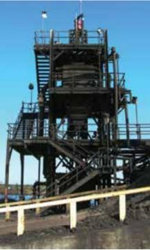
CrossFlow Separator installation for the recovery of heavy mineral.
